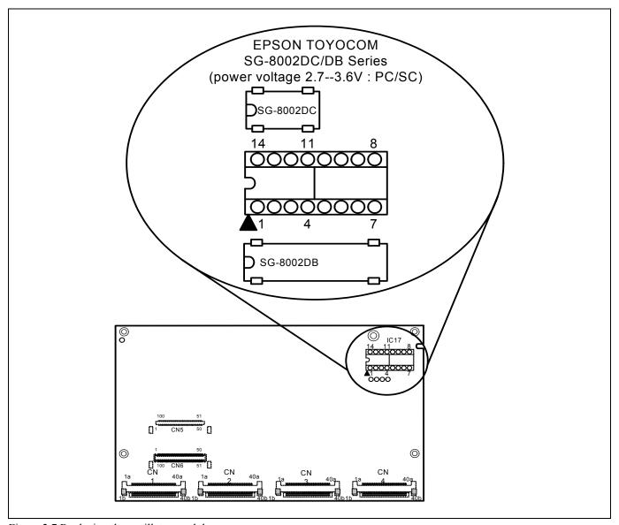
Figure 2.7 Replacing the oscillator module
